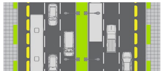
Camellón de mayor de 3m
